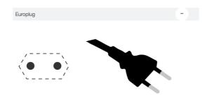
The **europlug (or plug type CEE 7/16)** can be used in most parts of Europe with the exception of the United Kingdom, Ireland, Cyprus and Malta. It has no protective conductor, which is why it is not protected against polarity reversal. Its contacts have a diameter of 4 mm and are placed at a distance of 19 mm.
